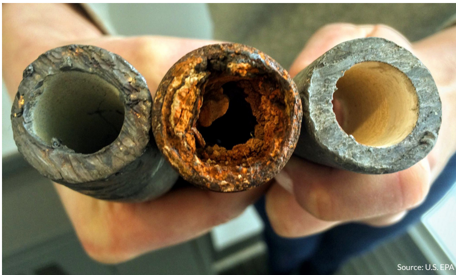
Left to right: a lead pipe, a corroded steel pipe, and a lead pipe treated with anti-corrosion material.
